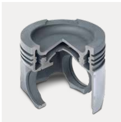
Forged, double-friction-welded monoblock steel piston
